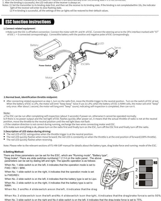
When No. 3 and No.4 slide switch are on the right, it indicates that the drag brake force is set to 100%.
