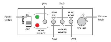
Power switch: To control the whole sound unit,
