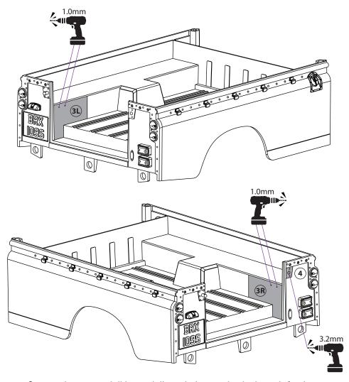
8. Use the 3.2mm drill bit to drill one hole completely through for the alum tailgate latch pin as indicated.
