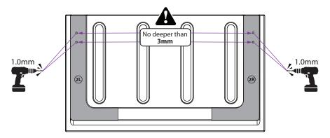
3. Attach the sticker guide to the outer side of the tailgate, aligning it with the tailgate edges. Drill four 1.2mm holes for the upper hinges at the marked locations. Drill one 1mm hole at the indicated location for the latch. Drill each hole no deeper than 3 mm to prevent breaking through.
