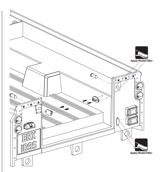
9. Secure the alum bed anchors to the rear bed using four ST1.2x4 screws. Remove the plastic tailgate latch pin and replace with the two alum tailgate latch pins.
