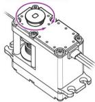
(6) Pull the switch button backwards to engage the locking mechanism.
