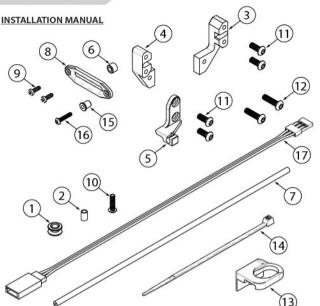
(1) This kit comes with a switch button for holding and releasing the knob Parts Included: Qty. to keep the spool engaged or (1) Pulley disengaged. (2) Pivot Tube (3) Winch Mount A (4) Winch Mount B (5) Tube Retainer (6) Nylon Washer (7) Routing Tube (8) Winch Lead
