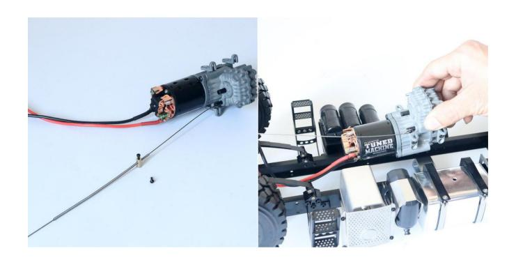
Put on the cable, fasten the cable screw with proper force, and ensure the sheath fastening passes through smoothly
