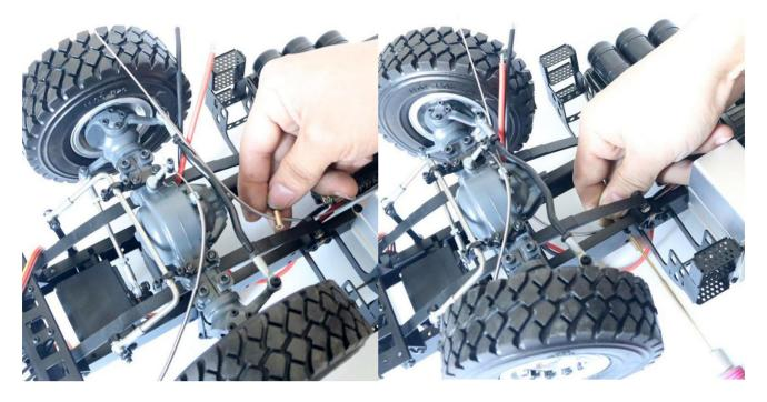
The cable passes through the cable seat
