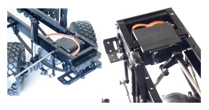
Install the variable speed steering gear (the steering gear needs to be purchased separately)
